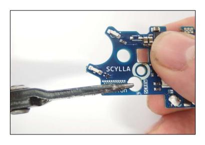
Separated board for instalation into the Krytac gearbox V2 and G&G G2.
