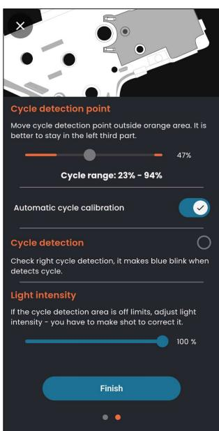
**Automatic cycle calibration** sets cycle detection point when error 103 appears.
