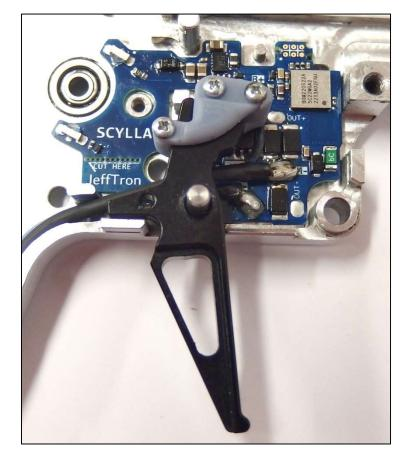
Check the sector gear height. Gear must not touch the optical sensor!
