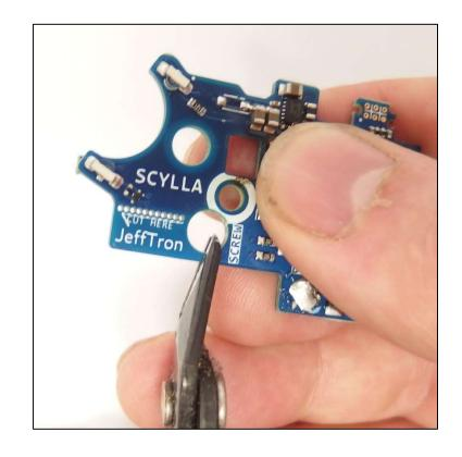
Put pliers near the drilled line and move the board up and down until it breaks of from the rest of the Scylla.
