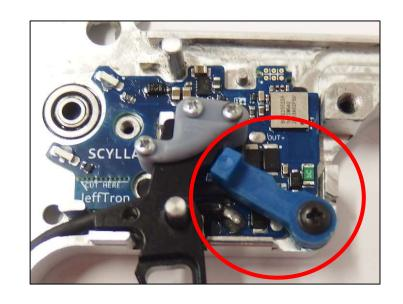
**electronic safety** to block firing, when is trigger pulled on Safe position.
