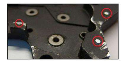
If your gearbox has high screw mounting, cut it off to flat surface.
