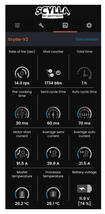
Semi cycle time: Time between motor start and a piston release.
