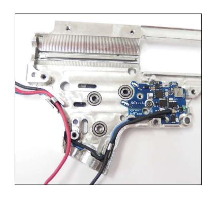
Wires to front: Red motor leads to the left hole and to the battery leads to front, it could be disconnected in the middle.
