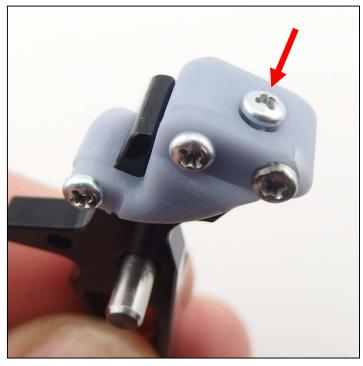
Make sure adapter will not hit sector gear teeth, otherwise grind the adapter to fit better on the trigger
