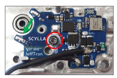
**too low**, move the sensor slightly **right** to be further from the sector gear or clean the sensor.
