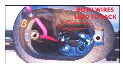
Connect the black wire first. Keep in mind the right motor polarity!
